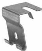
For trapeze hung QUICK TRAY PRO™ installations. Use with 1/4- or 3/8-in. threaded rod; obtain locally. Poly grommet retains tray in slot-unsnaps to detach one side of tray for loading cables. Corrosion-resistant pre-galvanized finish.
