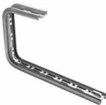
For QUICK TRAY PRO installations under ceiling or overhangs. Use with tray widths up to 12 in. (305 mm). To secure tray to bracket, use one QTPSSW3/QTPSSW3BLK Splice Washer and one QTPBNWK/QTPBNWKBLK Splice Kit on sizes up to 8 in. (203 mm); use two on 12-in. (305-mm) trays. Can be stacked for multi-level tray installations. Corrosion resistant plated finish.
