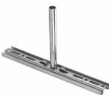
Use with up to 1/2-in. threaded rod (obtain locally). Only one rod needed to suspend tray. Snap-on attachment holds QUICK TRAY PRO cable tray secure without nuts and bolts. For use with 4- to 24-in. (102- to 610-mm) tray widths. Can be used for multiple-level installations; 1/2-in. threaded rod recommended. Corrosion-resistant plated finish.
