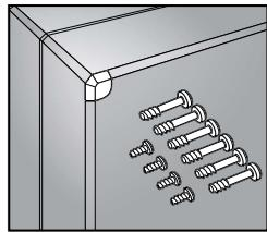
Hardware Kit includes six self-tapping, stainless steel cover screws, four self-tapping plated panel screws and six removable plastic caps that fit over the screws to provide tamper resistance as well as a clean aesthetic appearance. This kit is offered as a replacement kit for lost or damaged hardware originally furnished with the enclosure.
