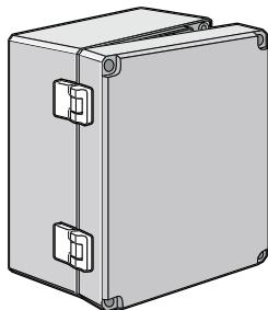
Hinge Kit includes two polyamide hinges, eight M4 self-tapping, plated screws, eight flat washers and drilling templates. Use on all QLINE™ D enclosures. Hinge Kit meets Type 4 requirements.
