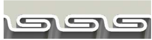
Interlocked Design 1-1/2" through 4" with no bonding wire
