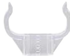
LAMP SUPPORT BRACKET FOR 5, 7, 9 & 13W G23 BASE LAMPS 3 HEIGHT ADJUSTMENTS: 17.5, 20.5 & 23.5MM UV STABILIZED • CLEAR D3940 (MUST BE USED WITH D3938)
