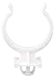
LAMP SUPPORT BRACKET FOR 2G11 TUBE RAISES LAMP 15.5MM SNAP IN BRACKET FOR 5.5MM CUTOUT D3958
