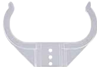
LAMP SUPPORT BRACKET FOR 2G11 TUBE 3 HEIGHT ADJUSTMENTS: 21, 24 & 27MM UV STABILIZED • CLEAR D3939 (MUST BE USED WITH D3938)
