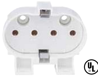
NON-DIMMABLE BALLAST 2G11 FLUORESCENT SOCKET 2G11 BASE BACK MOUNT HAS MOUNTING FEET 24MM ON CENTER PUSH-IN TERMINALS RATED 75W-600V D3936
