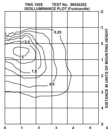
100W high pressure sodium lamp, horizontal lamp orientation, Footcandle values based on 10' mounting height, 9500 rated lumens Luminaire efficiency: 54.0%
