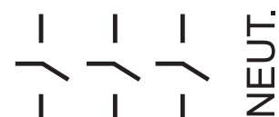
Four-wire SN, 240 Volts AC, No Fuse
