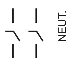
Three-wire SN, 120/240 Volts AC, No Fuse
