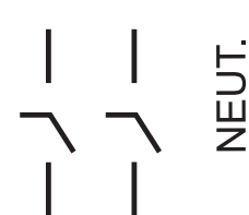
Three-wire SN, 120/240 Volts AC, No Fuse
