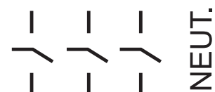
Four-wire SN, 240 Volts AC, No Fuse
