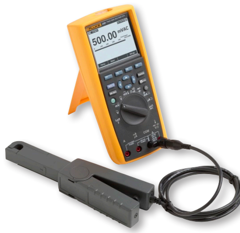
Figure 4: With the Fluke 289 DMM connected to the 80i-110s clamp, at 100 mV/A, a 5 amp reading displays 500 millivolts.
