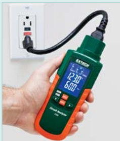
Tests 3-wire standard GFCI receptacles.
