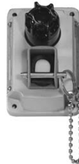
EDS factory sealed rocker arm push button control station—shows separate sealing chamber and device construction. Rocker arm has holes for lock.
