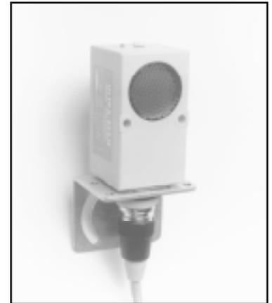
The Banner 925 Series ULTRA-BEAM is an economical ultrasonic sensor with relay output and a sensing range of 20 inches to 20 feet (0,5 to 6 meters). ULTRA-BEAM 925 Series sensors are ideal for long-range proximity requirements which fall beyond the limits of photoelectric response, and are the solution for many applications which require reflective sensing of non-reflective materials. Popular applications include bin-level sensing/control and presence sensing of transparent materials.
