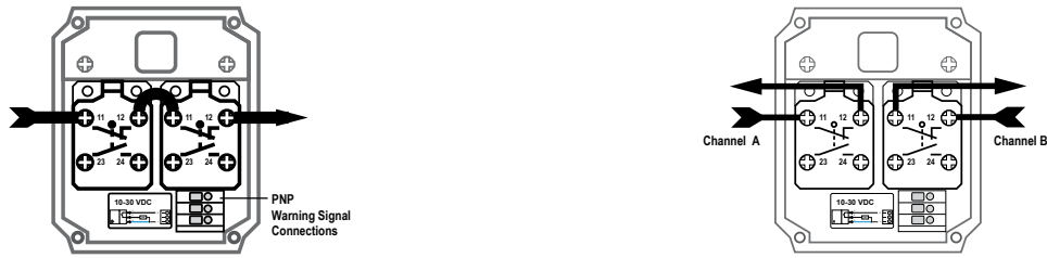
Figure 7. Wire the two switch contacts in series or independently, as described below
