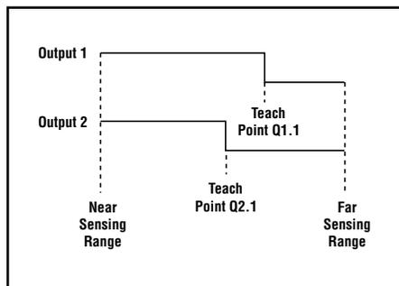
Figure 4. Each discrete output has its own limit for background suppression
