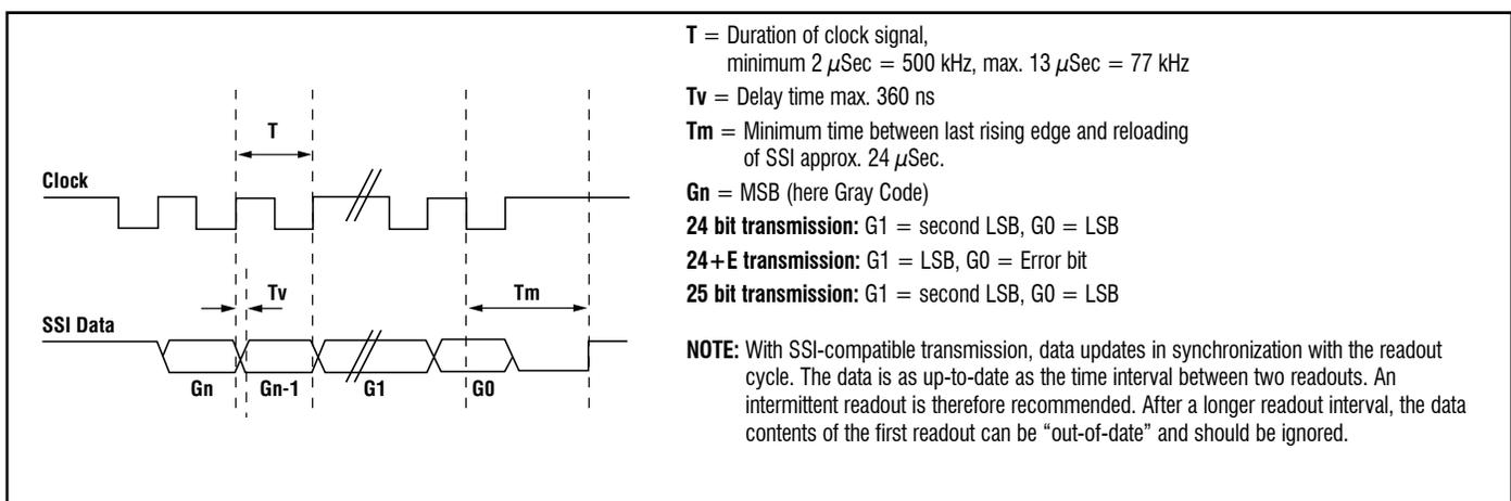
Figure 11. SSI-compatible interface timing
