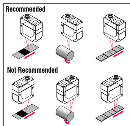
Figure 10. Sensor orientation for typical targets
