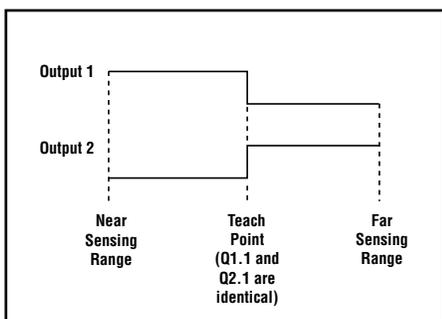
Figure 5. The two discrete outputs share identical limits for background suppression, but are complementary
