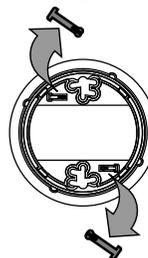
Close Door. Insert Pin in Holes through alarm and Battery Drawer
