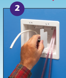
2 Tighten mounting wing screws to pull the box securely against the wall board (up to 1-1/2"). See Photo B at right. Insert voltage separator if installing power and low voltage Class 2 wiring.
