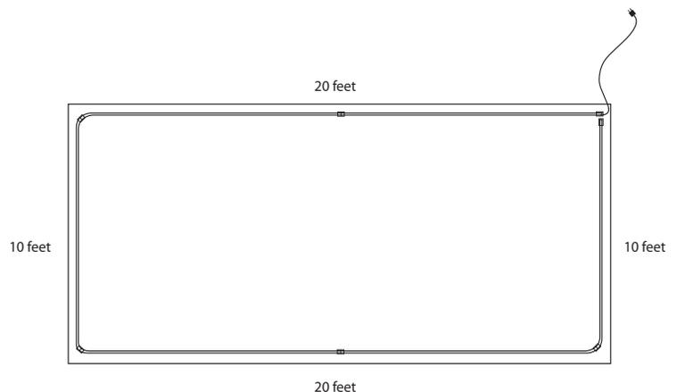
Consider using shorter length kits to build longer custom lengths. If one section should fail, a kit can be replaced (which maintains UL Listing) versus repairing a section, which voids UL.
