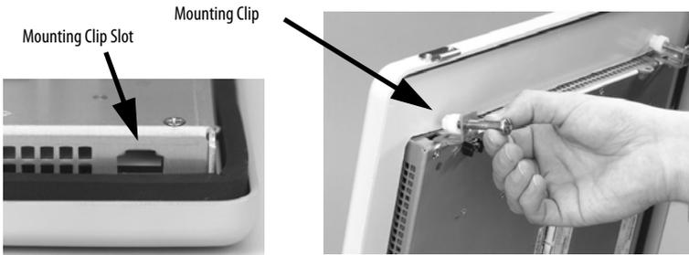
5. Tighten the mounting clip screws by hand until the gasket seal contacts the mounting surface uniformly.
