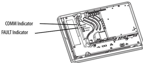
When the terminal starts, the fault indicator should be off, except for a few brief flashes, and the comm indicator on. If the indicators remain off, the power supply or logic module has failed. Check the power cable. If the power is not within range, replace the power supply. If the power is within range, replace the logic module. After a successful startup, both indicators are off and controlled by the application running on the terminal.
