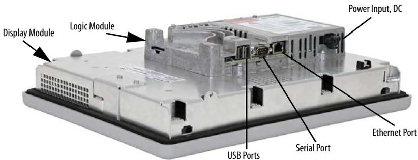
Attach the logic module and communication module to the display module before panel installation. See the instructions shipped with each module.
