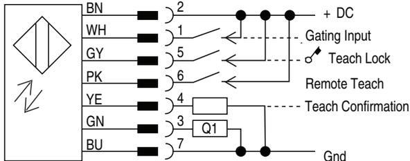
The control input (pin 5) can be used to lock the ColorSight pushbuttons by connecting it to the +DC (18...28V DC). When working with the sensor in remote teach, we recommend the use of pushbutton lockout to prevent accidental tampering of the configuration.
