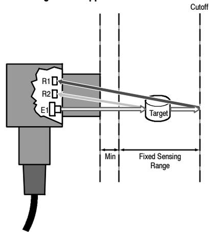
The gap between the target and background will vary with the shape and reflectivity of the target. This variance is known as the suppression quality and can be determined by the response curves shown for the sensor.
